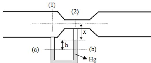
$$H_1 = H_2 \quad \text{ou} \quad z_1 + \frac{P_1}{\gamma} + \frac{v_1^2}{2.g} = z_2 + \frac{P_2}{\gamma} + \frac{v_2^2}{2.g}$$
