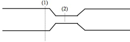
$$z_1 + \frac{P_1}{\gamma} + \frac{v_1^2}{2.g} = z_2 + \frac{P_2}{\gamma} + \frac{v_2^2}{2.g} \Rightarrow \frac{v_2^2 - v_1^2}{2.g} = \frac{P_1 - P_2}{\gamma}$$
